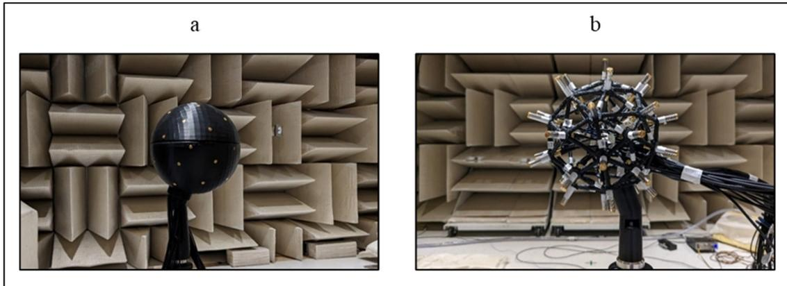
Figure 4.4 Picture of the a) rigid 36-microphone SMA and the b) open wire frame 36-microphone SMA during the experimental measurements
