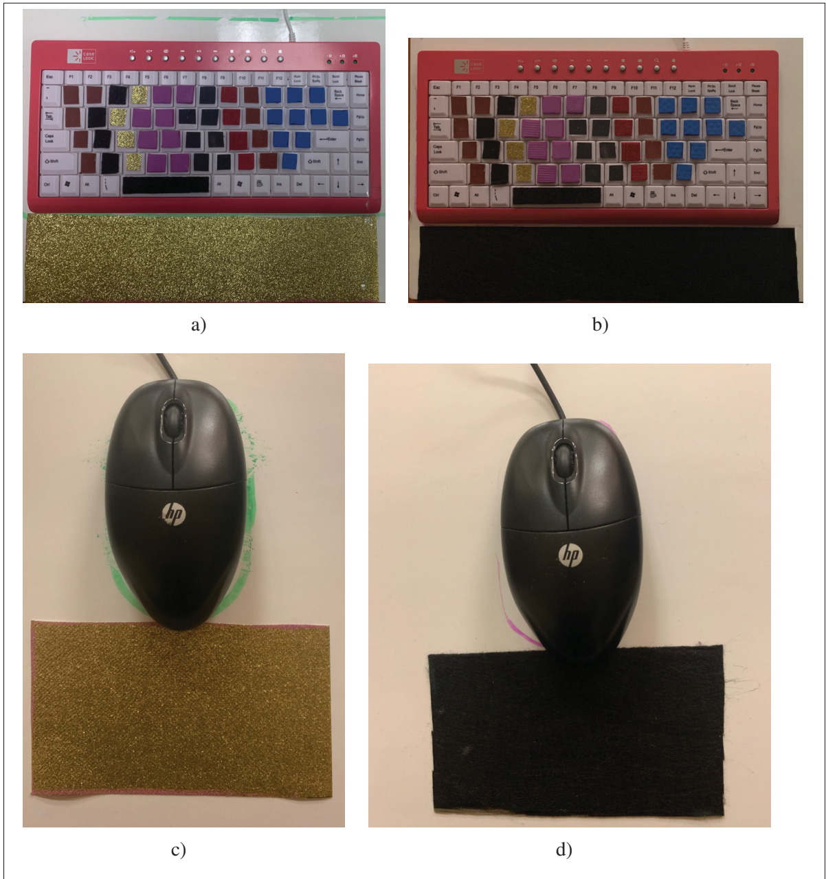
Figure 2.5 Haptic sketches: a) palm rest with sandpaper 120-grit, b) palm rest with fabric cotton, c) mouse pad with sandpaper 120-grit, and d) mouse pad fabric cotton
