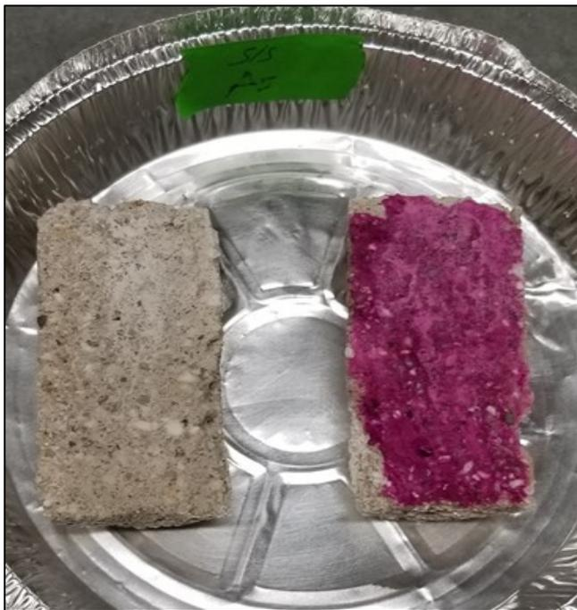
Figure 3.15 S/S sample stained with the phenolphthalein solution (NC/NL scenario)
