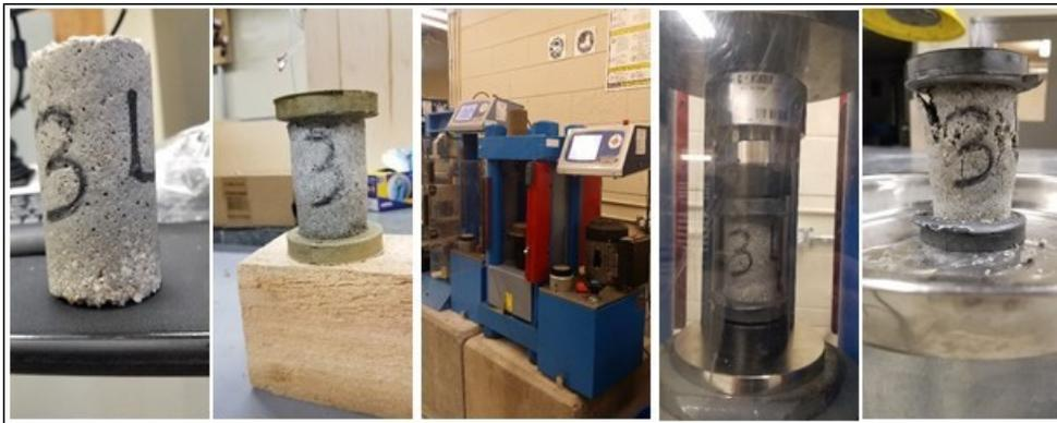
Figure 2.12 Uniaxial compression test on a cylindrical sample
