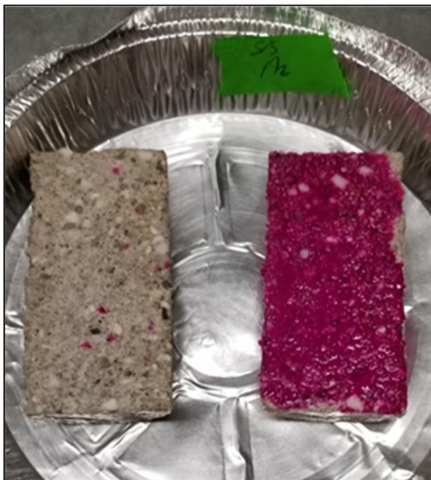
Figure 3.16 S/S sample stained with the phenolphthalein solution (L scenario)
