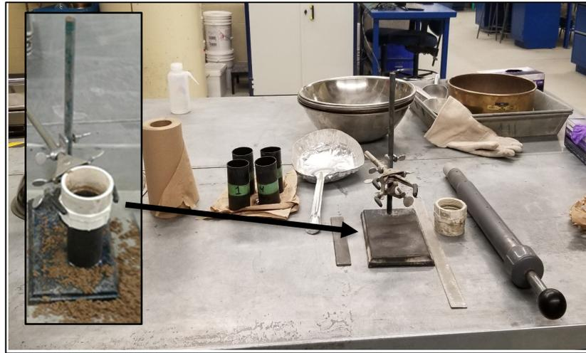
Figure 2.11 Compacting tools used to prepare S/S samples
