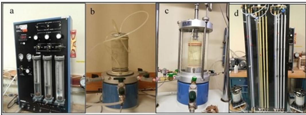
Figure 2.13 Equipment of triaxial cell: a) control panel, b) sample placed on the base of the cell, c) the sample under the test, and d) the hydraulic conductivity panel (burettes)
