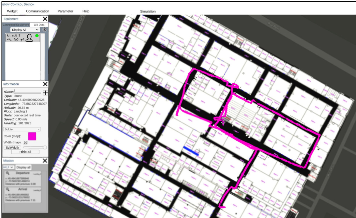
Figure 2.9 Visualizing a sample test trajectory on GCS platform: map of ÉTS with reference path
