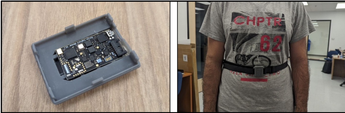
Figure 4.1 Different views of the ibNav 6.1 sensor. The board itself on the left and the sensor on the user's chest on the right
