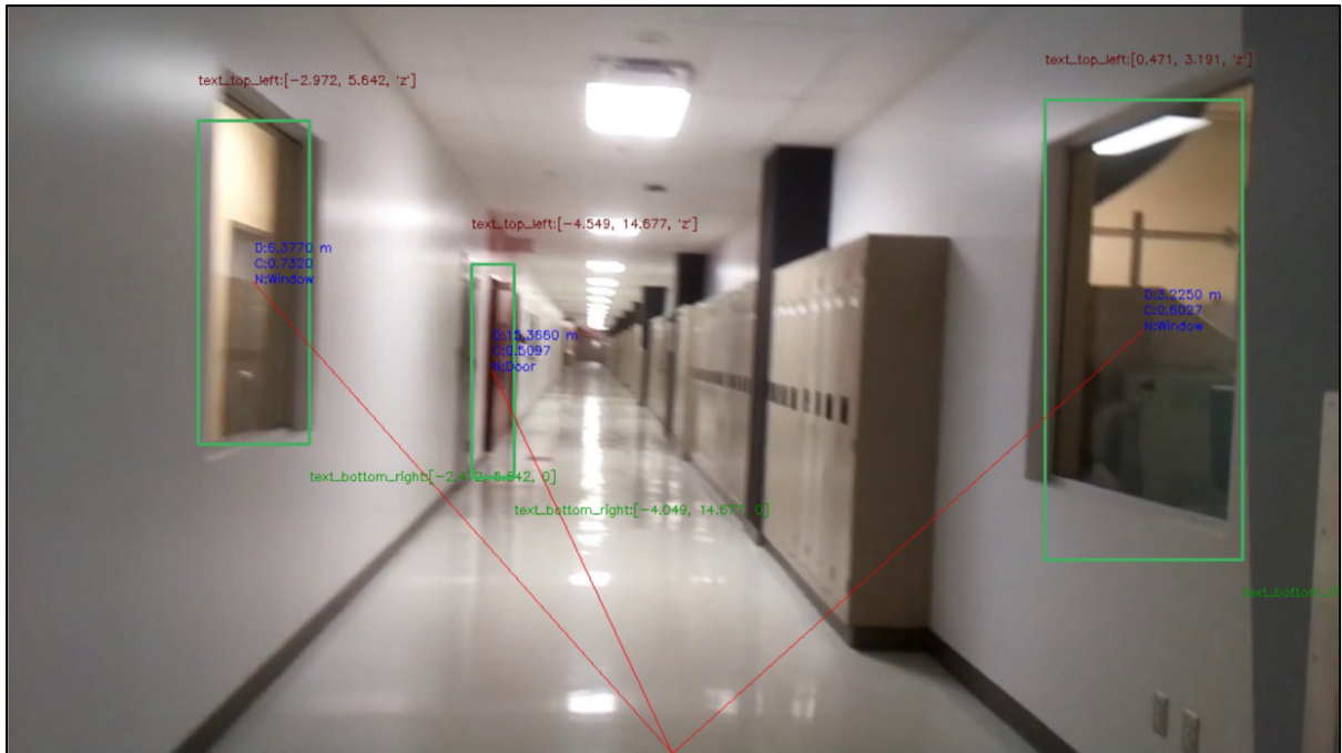
Figure 1.13 Depth measurement and object detection using camera
