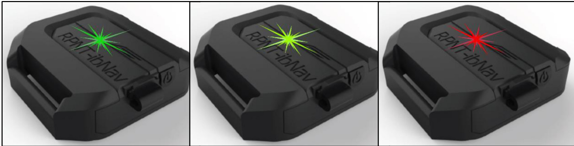
Figure 1.5 LED status of different battery levels of ibNav 6.1
