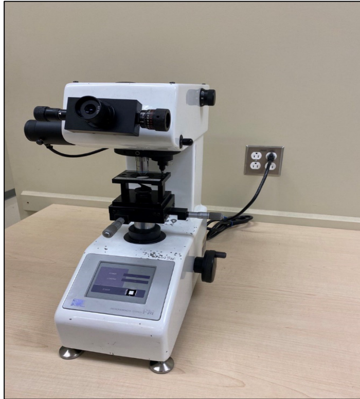
Figure 2.4 Future-Tech FM-1 microhardness tester
