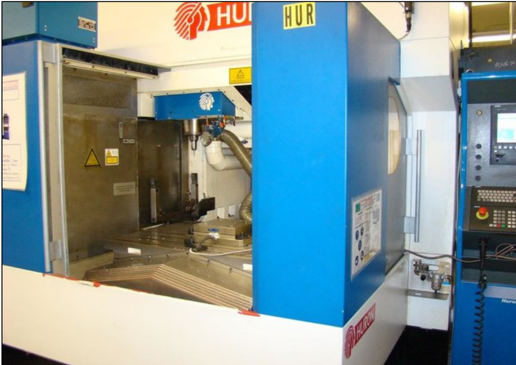
Figure 2.5 Three-axis CNC HURON K2X10 machine tool Taken from Slamani, Gauthier and Chatelain (2016)
