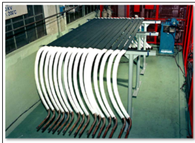
Figure 1.6 Picture of stator bars Taken from OMICRON (2023, p. 30)
