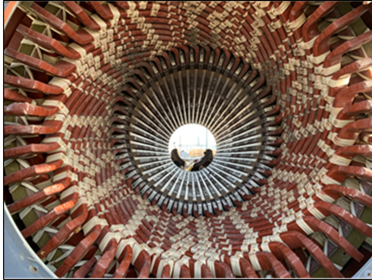
Figure 1.4 Picture of a stator winding of a 230 MW turbo generator Taken from Lachance & Oetl (2020, p. 435)
