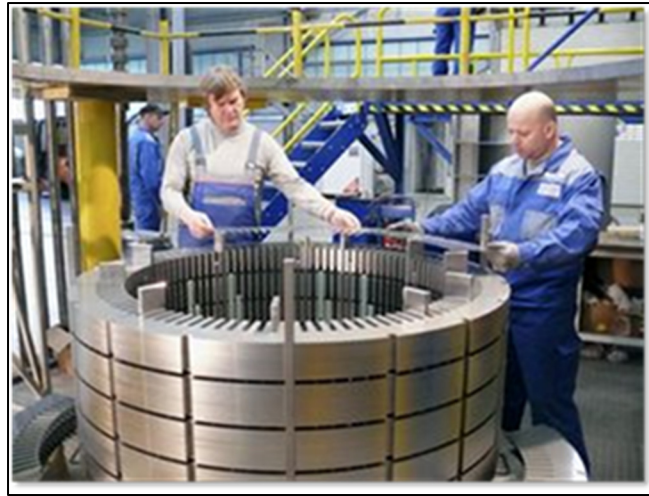
Figure 1.3 Picture of a magnetic core being assembled Taken from OMICRON (2021, p. 2)
