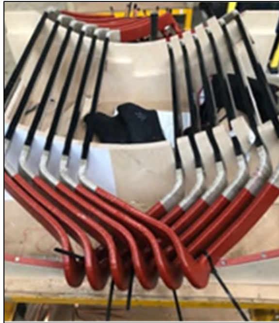
Figure 1.5 Picture of stator coils Taken from OMICRON (2023, p. 30)
