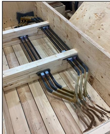
Figure 4.2 Picture of the three stator coils used as test specimens
