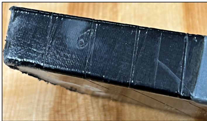
Figure 7.16 Picture of the suspect fault area of coil 19
