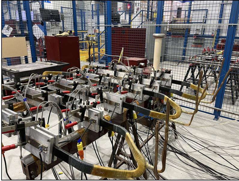
Figure 4.6 Picture of the test bench for the voltage endurance test
