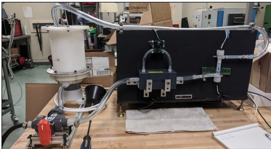
Figure 2-3 Flow rig to measure the pressure drop of the foam samples
