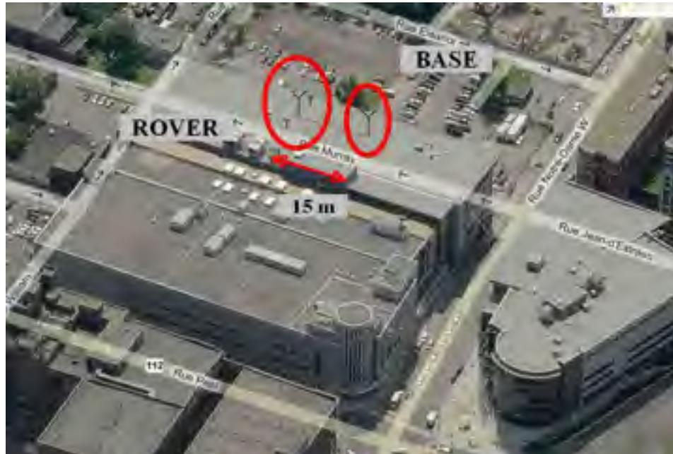
**Figure 4.2 Static configuration of the antennas on the ETS rooftop.
