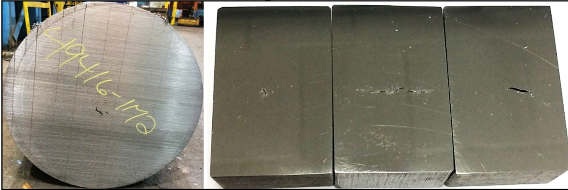
Figure 2.2 Porosities observed at the centerline of H13 bars on a transverse cut
