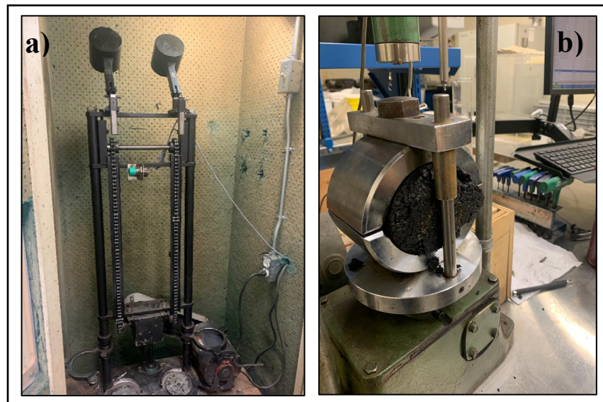
Figure 3.27 Marshall compaction. a) Marshall compactor, b) Marshall specimen during the test
