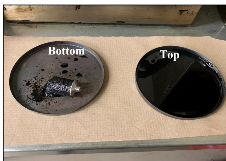
Figure 4.2 The bottom (left) and top (right) of the tube for the modified bitumen with K SW B lignin after the first grinding process
