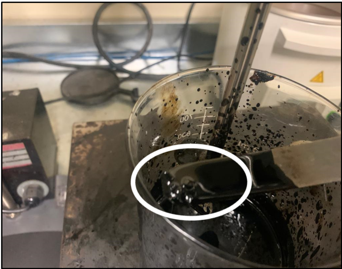
Figure 4.5 A photo taken during the incorporation process of the HDI pellets by LSM showing the presence of pellets
