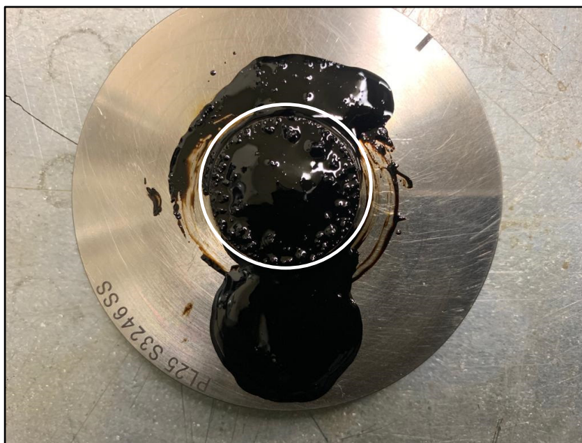
Figure 5.10 A photo shows the particles of HT SW A-modified lignin on the plate used for the DSR test
