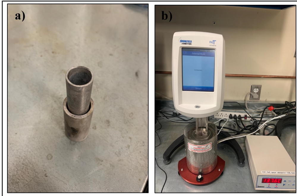
Figure 3.19 Brookfield Rotational Viscometer (BRV) test. a) BRV mold, b) BRV apparatus
