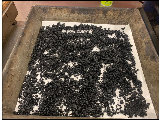
Figure 3.26 Loose HMA specimen used for G_{mm}
