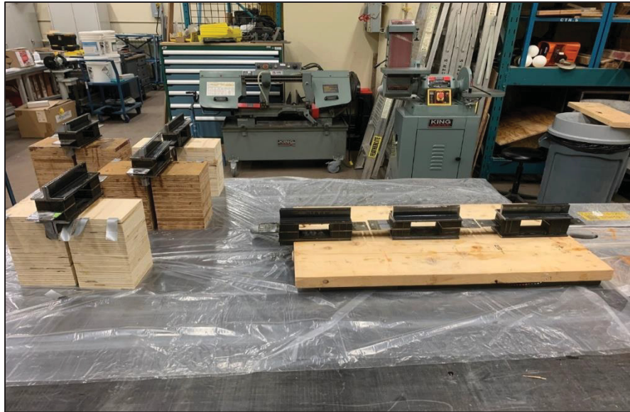
Figure 2.16 Gluing T-shaped plates to both sides of the original CHB samples by using Sika300 glue
