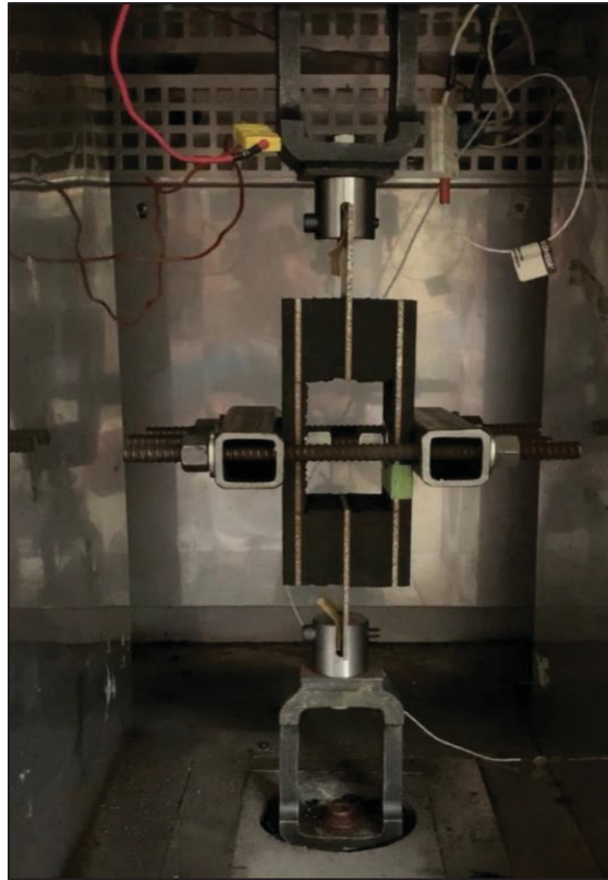
Figure 2.13 The Champlain Bridge sample with metal-box bracing system
