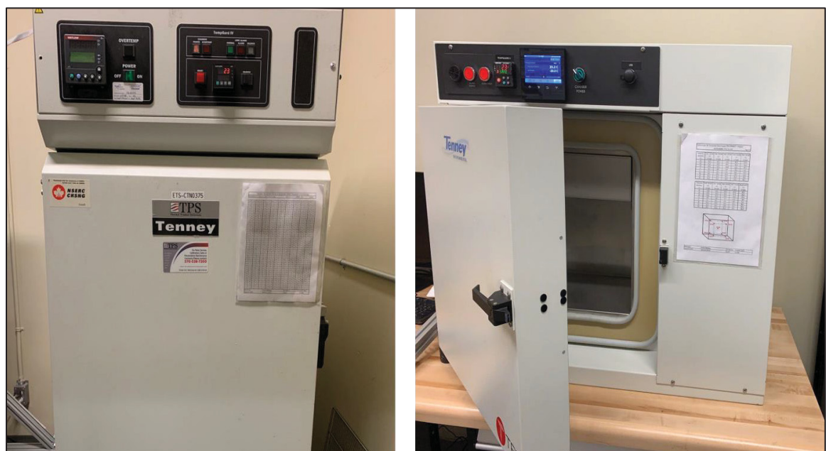
Figure 2.21 Freezer used to preserve specimens at -8^{\circ}\text{C} and -30^{\circ}\text{C} for long cold conditioning
