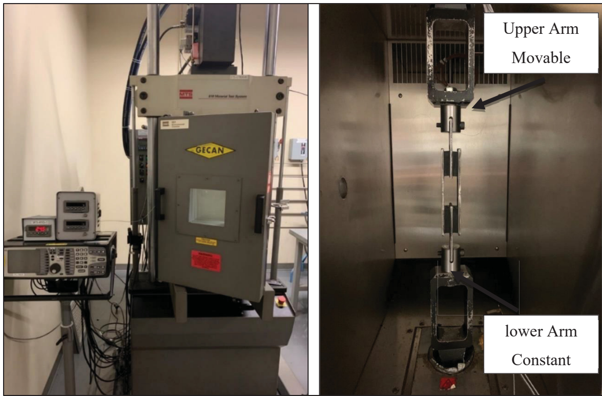
Figure 2.20 MTS Landmark 810 used in the shear tests
