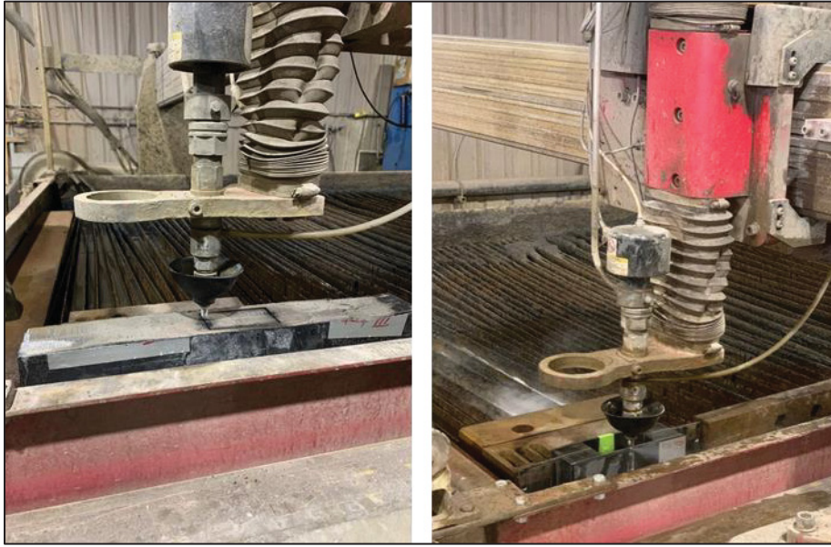
Figure 2.14 Cutting the Champlain Bridge bearings by water jet to make the quadruple samples
