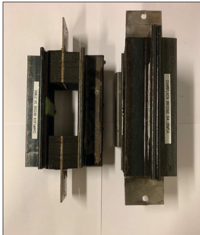
Figure 2.17 Specimens of CHB D4.27(left) and CHB D4.28 (right) with T-shape plate
