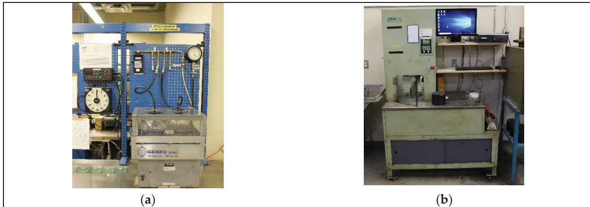
Figure 4.4 Determining HMA volumetric properties and compactability: (a) maximum specific gravity (Gmm) test; (b) shear gyratory compactor (SGC) device
