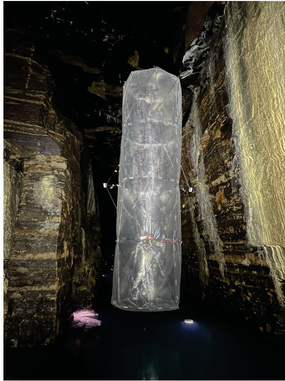
Figure 6.25 CAVERNAUTE flight above water at St-Léonard aquatic section. The two side motor pods equipped with their micro-lattices patches can be seen.
