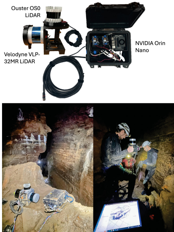
Figure 6.13 On top, a photo of the device with two LiDARs. Bottom left, is an in-cavern photo of the device with three LiDARs, and the bottom right is in use with remote SSH access with a rugged tablet.
