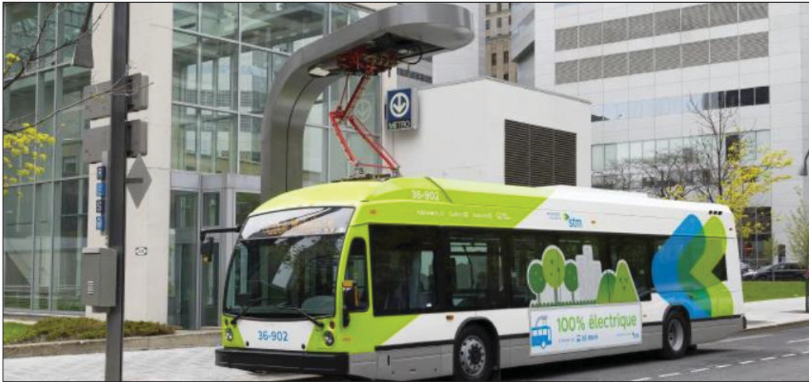
Figure 5.6 Fully electric bus with fast-charging station Adapted from: Ville de Montréal (n.d.a)
