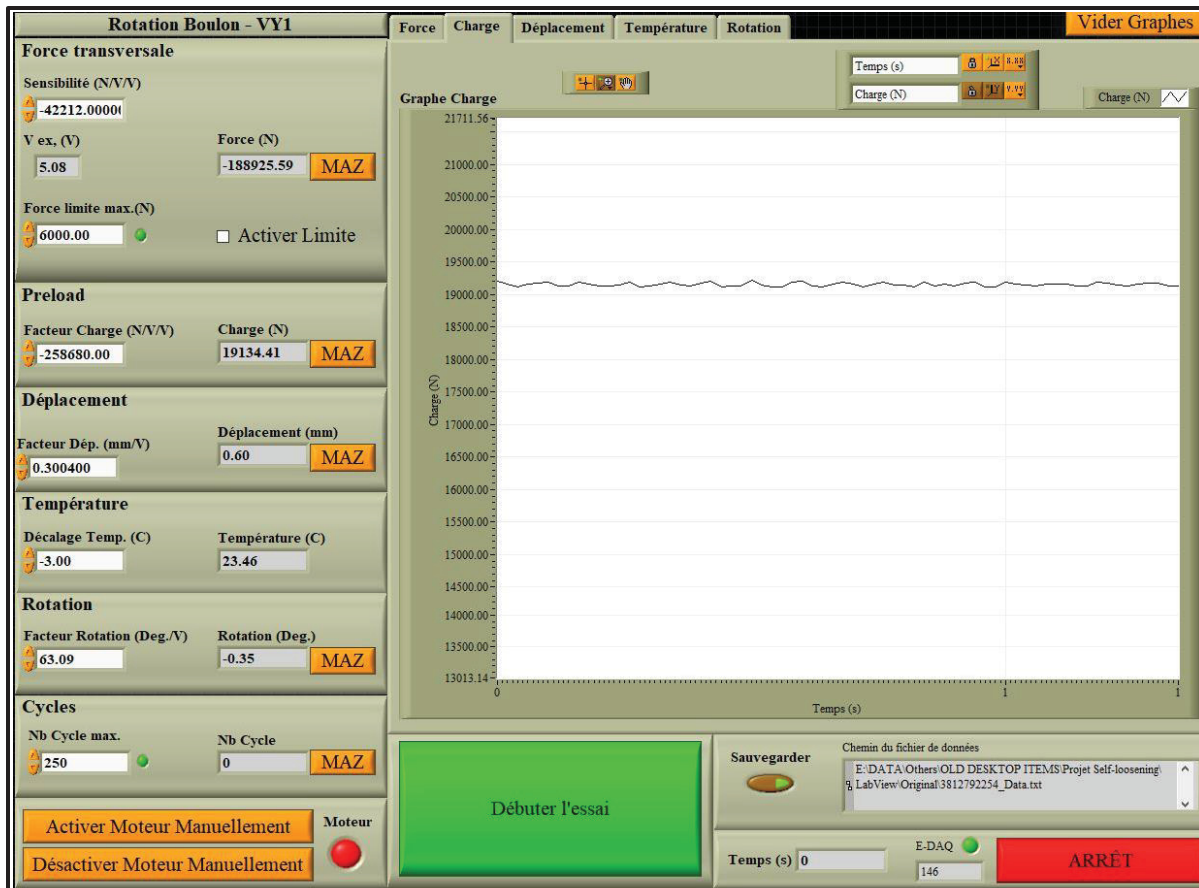
Figure 2.18 LabView user interface of the data acquisition system
