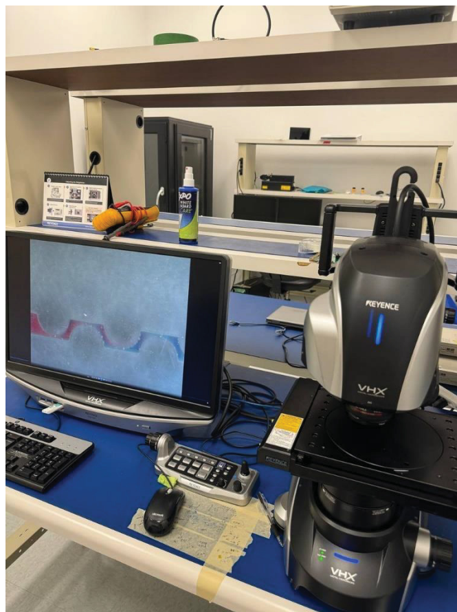
Figure 3.8 Digital microscope (KEYENCE, VHX-7100) from ETS university
