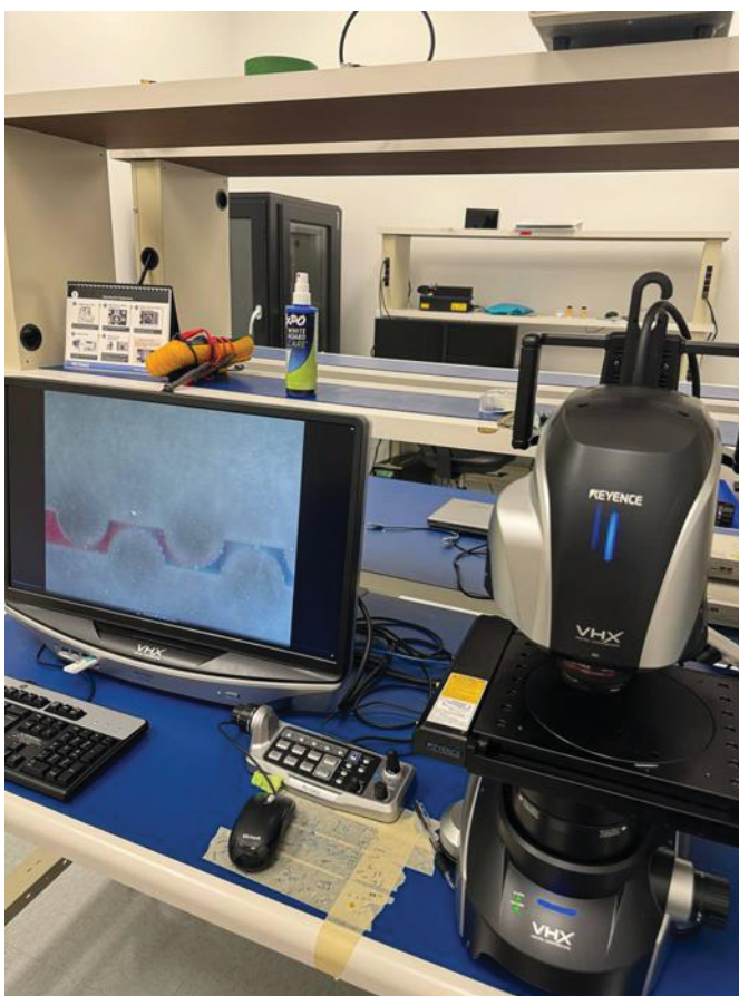
Figure 2.6 Digital microscope set-up for imaging milli mixers purchased from Keyence set-up
