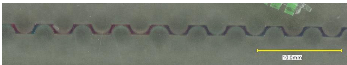
Figure 3.9 The picture of mixing blue and red dyes inside the PDM milli mixer with FRR=5 and TFR=120
