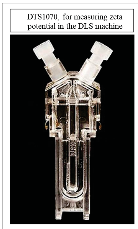
Figure 2.16 Capillary cells used in Zetasizer Nano pro for microelectrophoresis Taken from (Panalytical)
