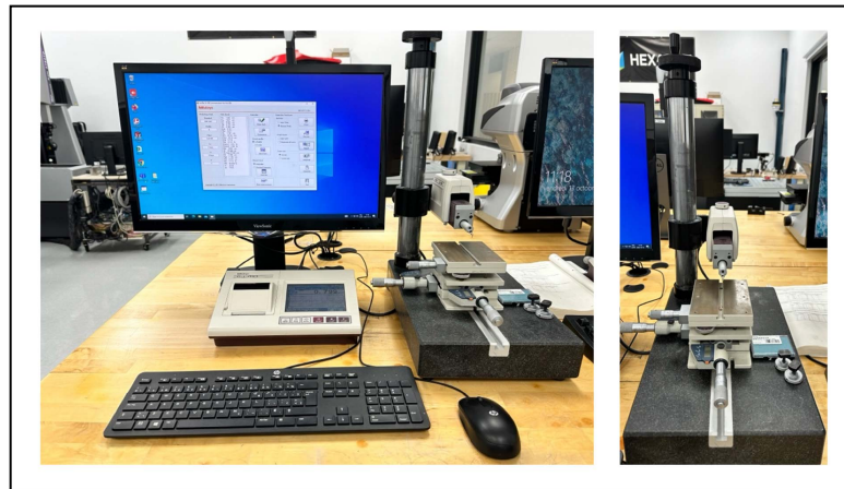
Figure 2.12 Mitutoyo SJ-410 surface roughness tester used for surface roughness measurement
