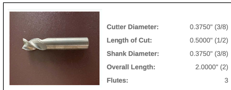
Figure 2.10 Cutting tool (3 Flute, Square - 40° Helix, Variable Pitch)
