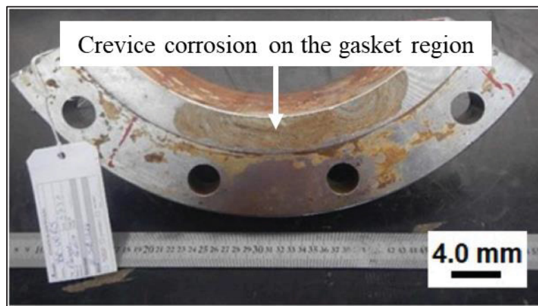
Figure 1.4 Crevice corrosion observed on the UNS S32760 SDSS flange face in the gasket region
