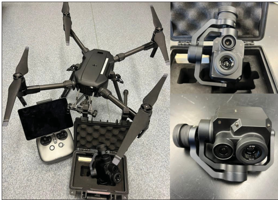
Figure 2.3 Images of the unfolded DJI Matrice 200 drone, its control remote, and the Zenmuse XT2 payload, pairing a visible camera and a FLIR T thermal sensor
