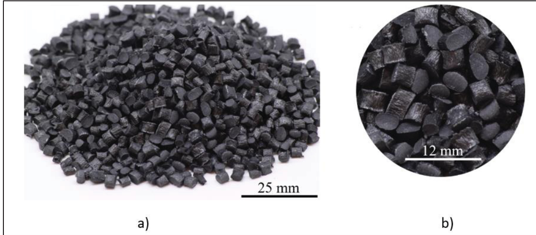
Figure 2.2 CF/PEKK-PEEK recycled pellets made from CF/PEKK pre-impregnated tape edge trims
