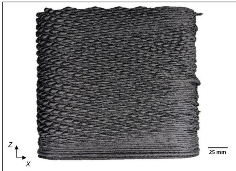
Figure 2.16 FGF box printed using parameters of Table 2.2 with the twice-recycled pellets (pellets obtained from shredded printed boxes)
