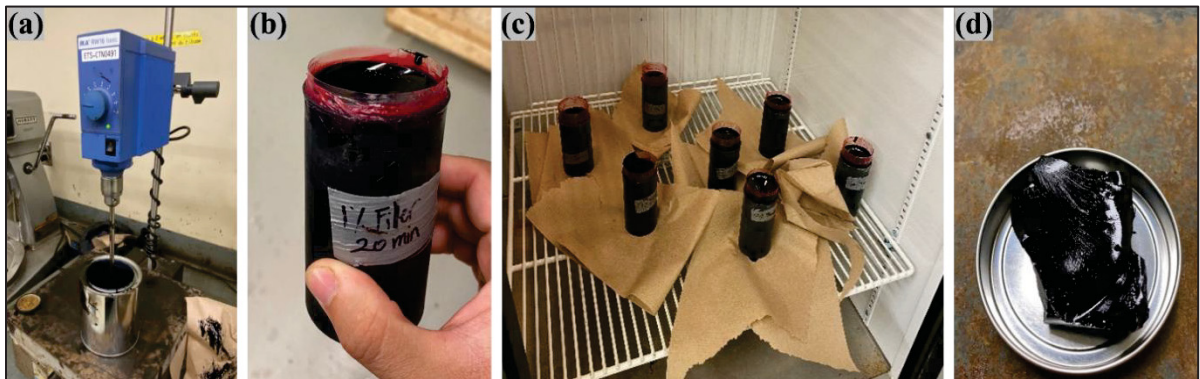
Figure 3.3 Sample Preparation Process for microscopic observations: (a) Mixing bitumen with Aluminosilicate and filler, (b) Mixed samples in the mold, (c) Samples placed in the freezer, (d) Breaking the frozen samples and ready for microscopic observations
