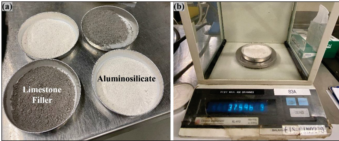
Figure 3.4 Preparation (a) and Measurement (b) of Aluminosilicate and Limestone filler Samples for Water Content Testing
