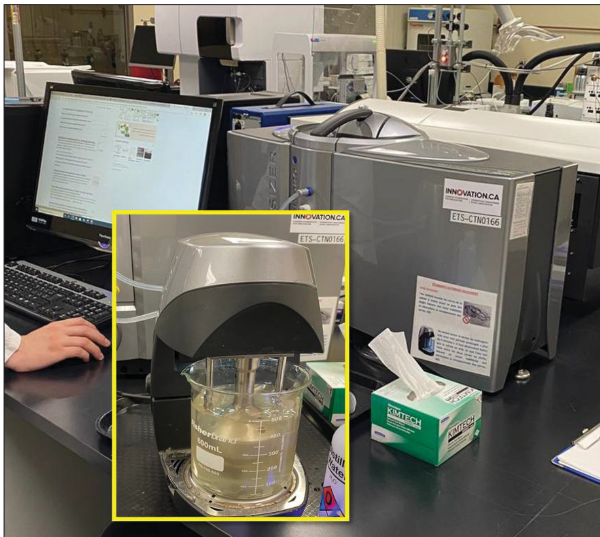
Figure 4.6 Experimental Setup for Laser Granulometry Test Using Mastersizer 3000
