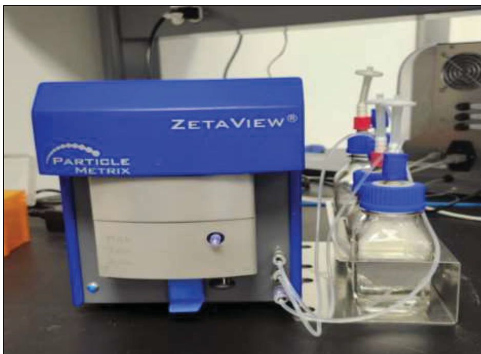
Figure 2.5 ZetaView PMX 120 nanoparticle tracking analyzer (Particle Metrix) used for measuring size distribution and zeta potential of extracellular vesicles (EVs) and synthetic vesicles (SVs)
