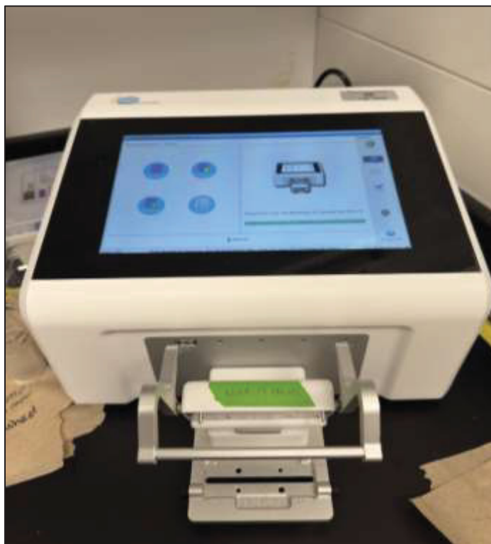
Figure 2.8 Flex S NanoGenerator system (Precision NanoSystems Inc.) used for the microfluidic synthesis of synthetic vesicles (SVs)
