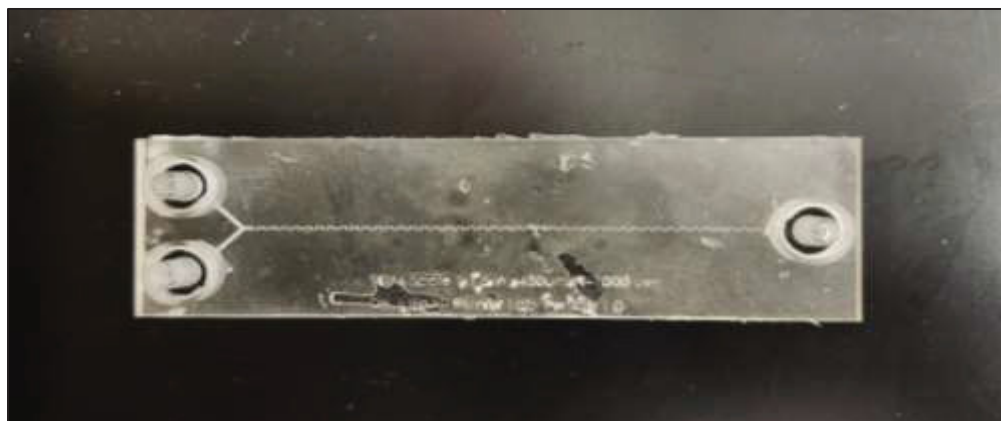
Figure 2.7 Polydimethylsiloxane (PDMS)-based microfluidic chip used for the synthesis of synthetic liposomes via passive mixing Originally developed by López et al. (2021)
