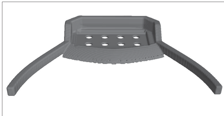
Figure 5.2 Render view of the Wave Dragon, showing the accuracy of the model
