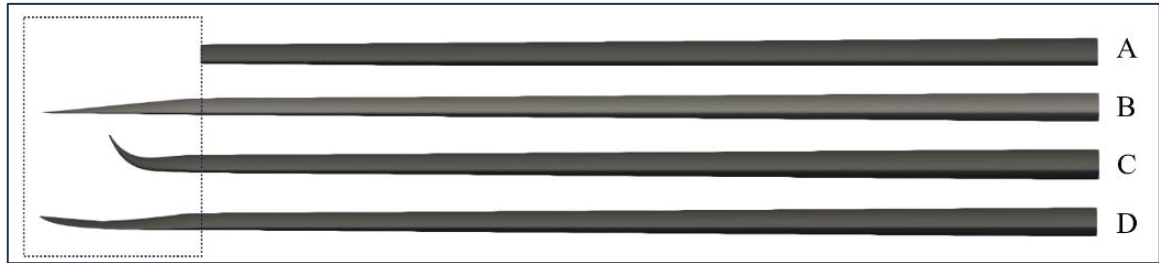
Figure 7.16 Wingtip configurations, A) baseline wing, B) proposed wingtip (flattened winglet), C) baseline wing with standard UAS-S45 winglet, D) Twist morphing wingtip
