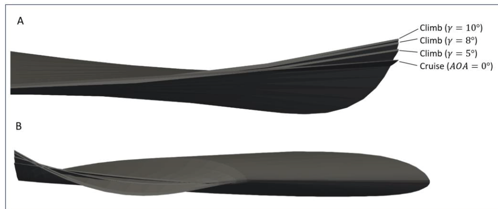
Figure 7.18 Optimum twist morphing wingtip configuration for four flight conditions: A) rear view, B) side view
