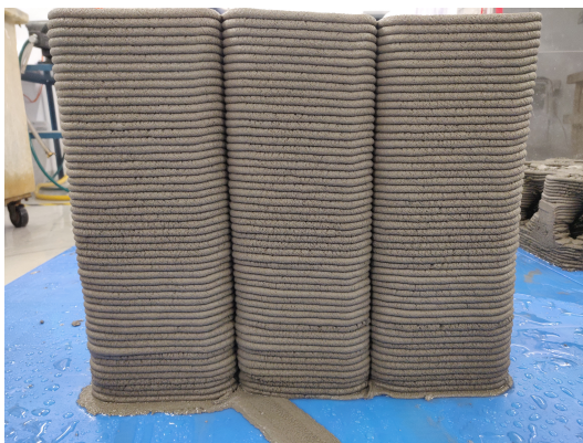
Figure 5.25 | Impression 3D du mélange LC3-1
