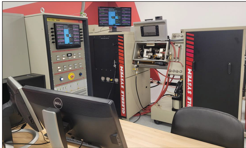
Figure 3.1 The thermomechanical simulator, Gleeble 3800 ® , used for the high temperature isothermal compression tests
