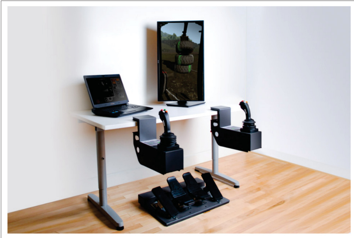
Figure 2.5 The Vortex Edge Simulator was used for collecting the dataset and training the reinforcement learning policy. To provide a close-to-realistic scenario, a mobile setup was installed, featuring a single vertical monitor, touch-sensitive operator console, and physics controls. While the operator uses external joysticks to provide signals to the actuators, in the RL setup, a Proximal Policy Optimization (PPO) policy maps the observation space to the required torque for each actuator
