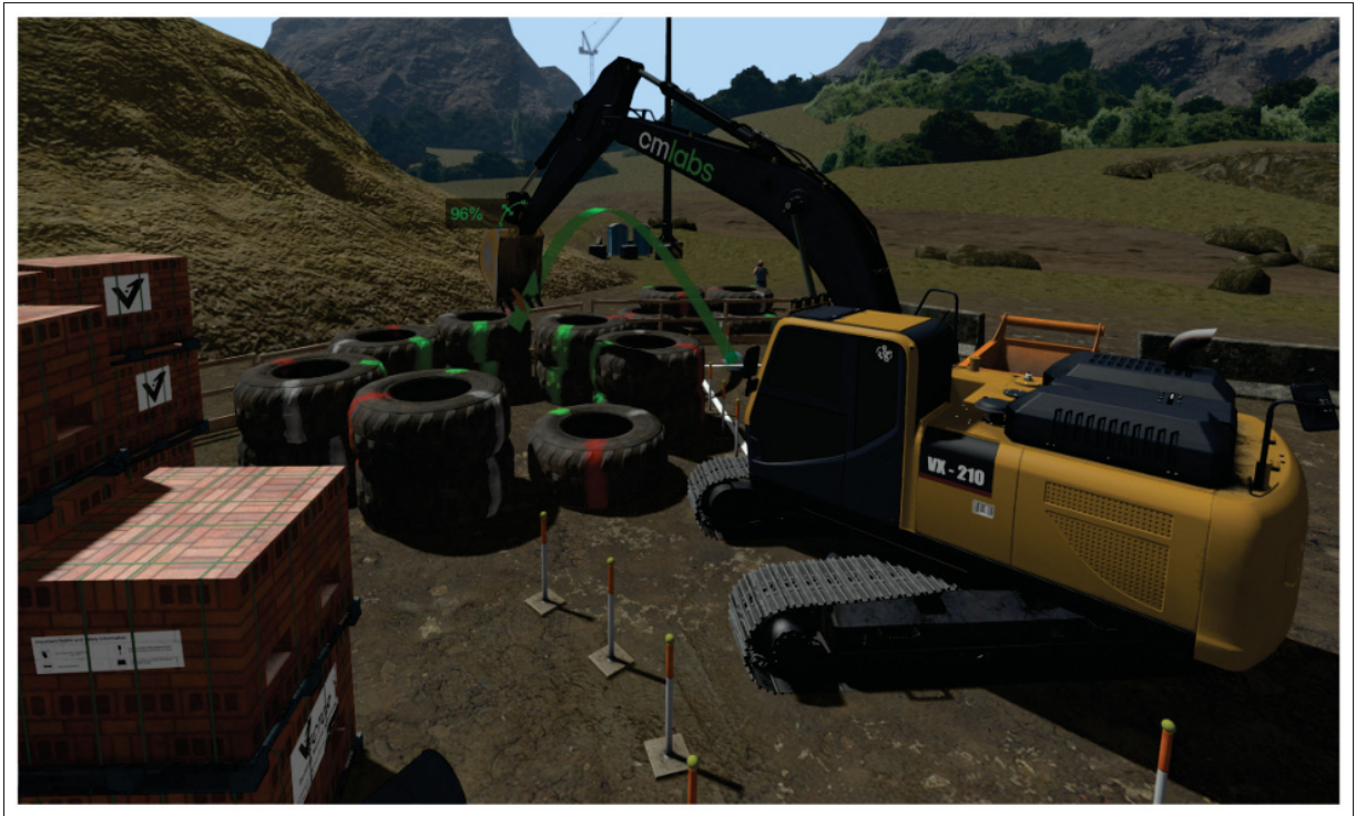
Figure 2.4 The Vortex Excavator environment presents a challenging, yet effective, tool for training users on the safe and efficient manoeuvring of the excavator while considering multiple external factors. The complex task requires precise coordination of multiple actuators while also accounting for the machine’s internal dynamics and various external infractions
