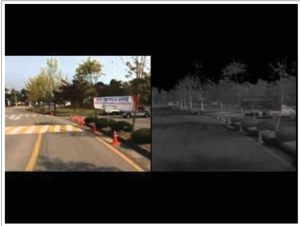
Figure 1.25 Example of Forward Looking Infrared (FLIR) image from Kaist Multispectral Dataset. The FLIR operates on the long-wavelength infrared (LWIR) spectrum Taken from Hwang et al. (2015)
