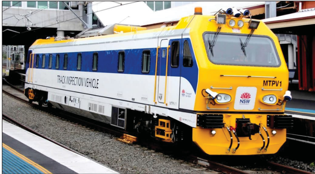
Figure 1.32 ROGER 800 Track inspection vehicle Taken from MERMEC (n.d.)
