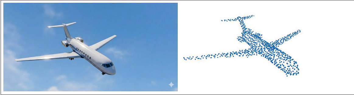
Figure 1.1 A 2D RGB image of an airplane (left) and its corresponding 3D point-cloud representation (right), illustrating the fundamental difference between dense pixel grids and sparse, unordered 3D coordinates
