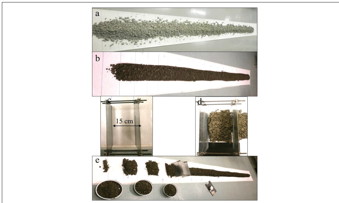
Figure 3.2 Probabilistic sampling : (a) dry longitudinal pile, (b) humid longitudinal pile, (c) sampling tool, (d) sample delineation, (e) sample extraction
