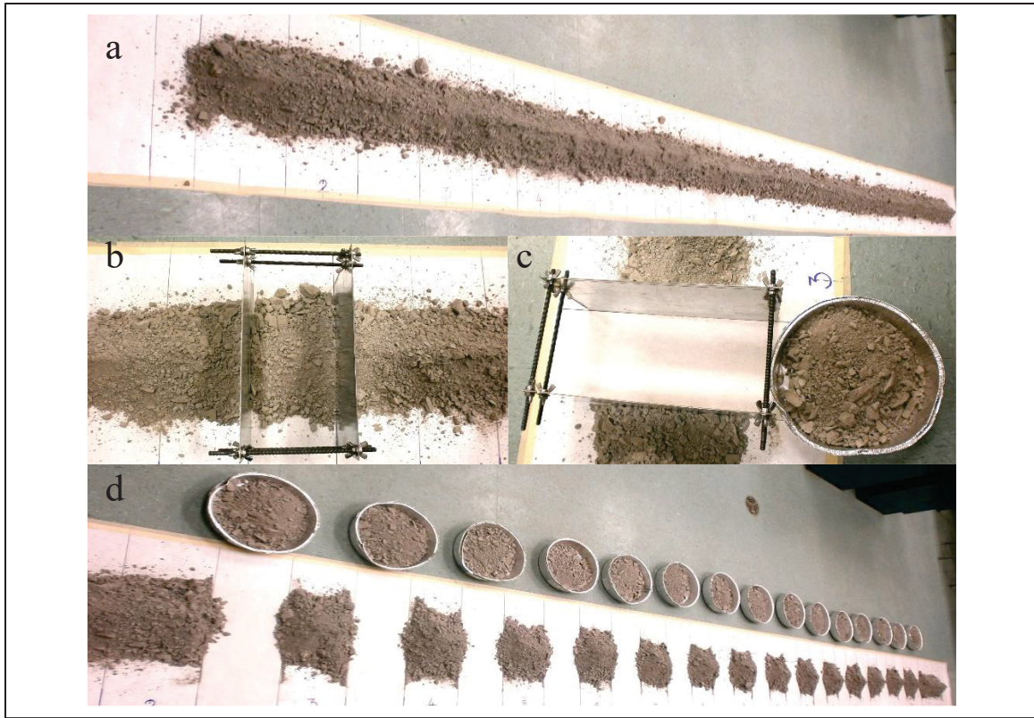
Figure 4.3 First stage of Probabilistic Sampling (PS I) : (a) elongated pile; (b) increment delimitation; (c) increment extraction; (d) extraction of 15 increments
