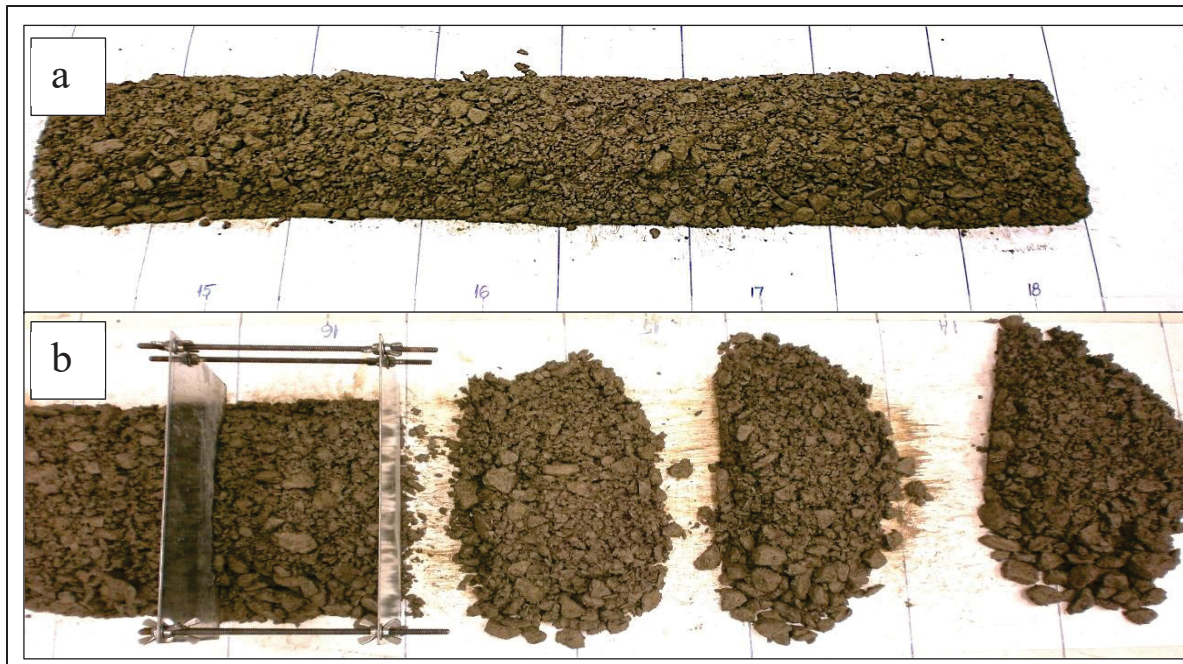
Figure 5.4 Second stage of probabilistic sampling (MPS-II): (a) 1D pile, (b) delineated and extracted increments
