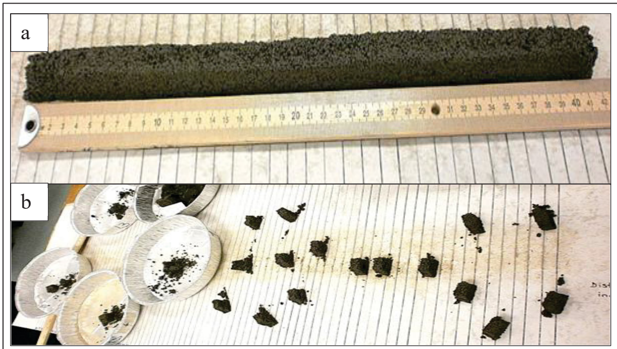
Figure 5.6 Fourth stage of probabilistic sampling (MPS-IV): (a) 1D pile, (b) delineate and extract increments on the line pattern
