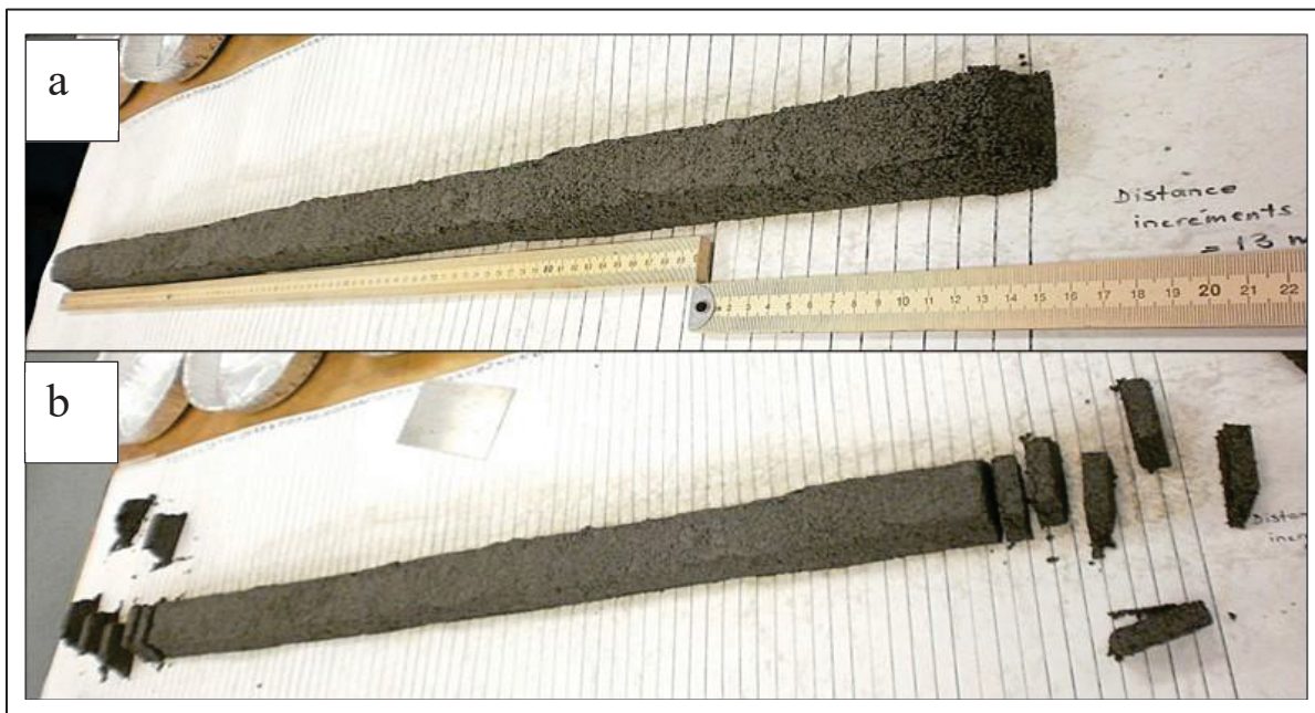
Figure 5.5 Third stage of probabilistic sampling (MPS-III): (a) 1D pile, (b) delineate and extract increments on the line pattern using an aluminum plate
