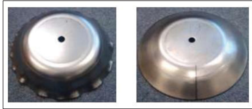
Figure 1.3 Wrinkling failure versus wrinkle-free forming in conventional spinning Reproduced from Wang (2011)
