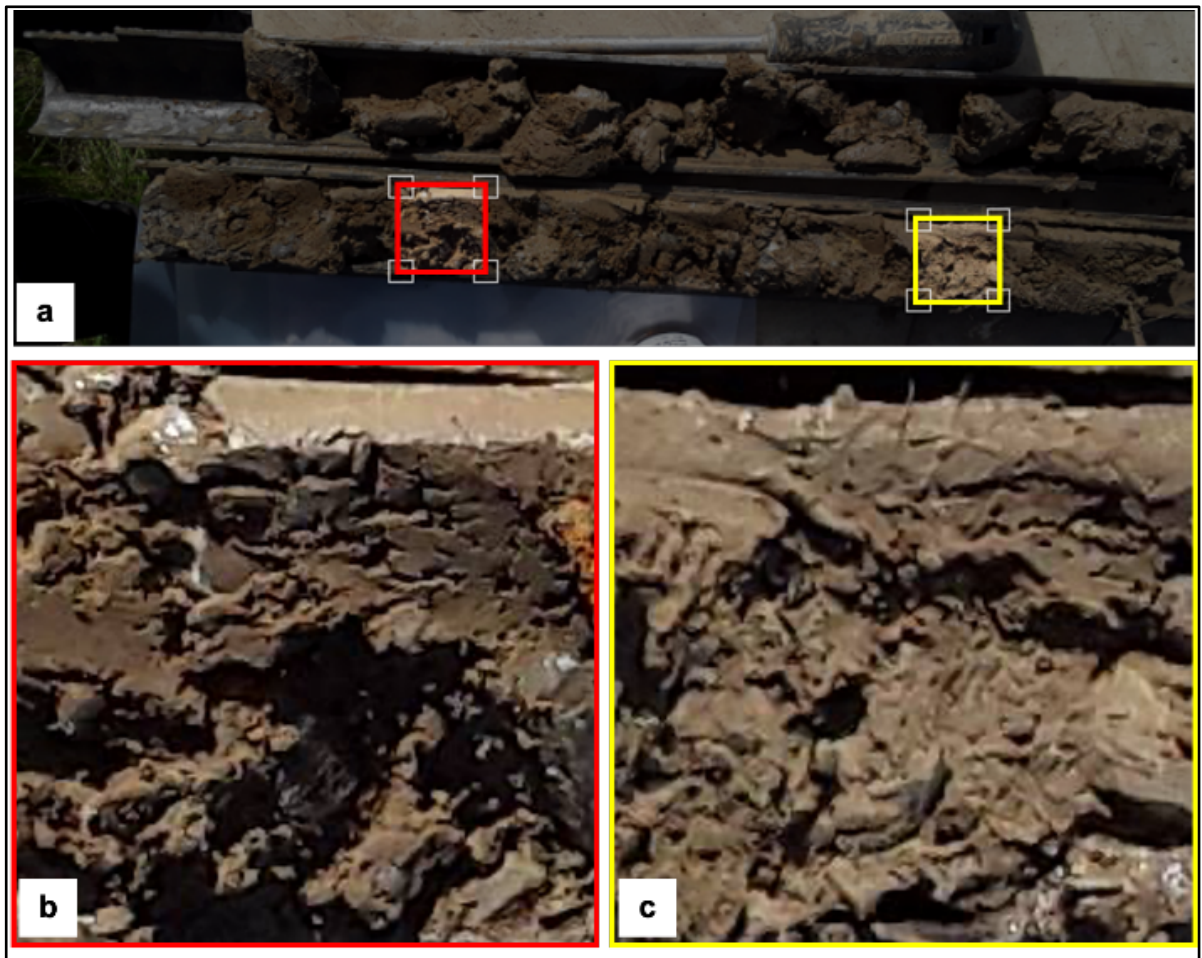
Figure 4.2 Example of split-spoon photograph subsampling and resizing with a) original image, and b) and c) selected subsamples cropped and resized to 299 \times 299 pixels
