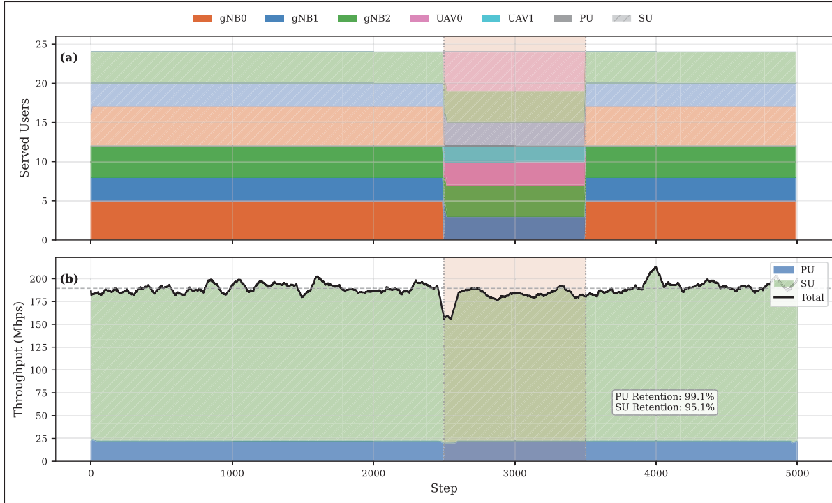
Figure 4.7 Disaster recovery: (a) user reassociation during outage, (b) throughput retention
