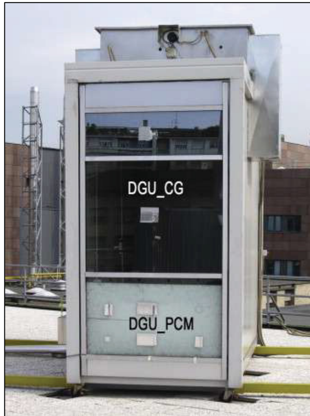
Figure 1.7 Test cells composing DGU with clear glasses and DGU-PCM taken from Goia et al. (2013, p. 444)
