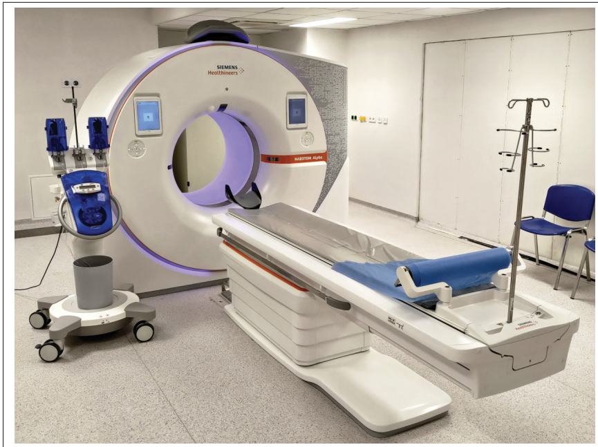
Figure 1.3 CT scanner featuring a patient table and a gantry that houses the rotating X-ray tube and detectors Taken from Tomas Vendis, 2024, Wikimedia Commons, CC BY-SA 4.0
