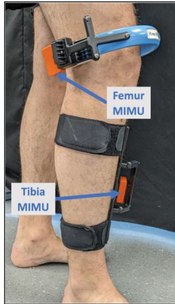
Figure 4.1 KneeKG attachment system with two Xsens MIMU attached on each of the two parts
