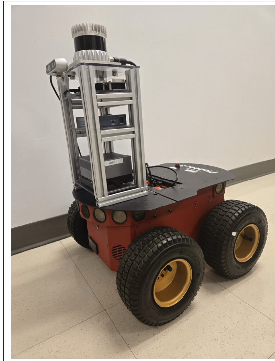
Figure 6.5 Modified Pioneer 3-AT
