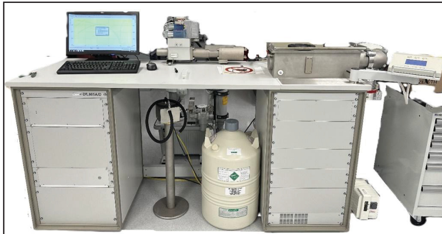
Figure 2-5 Dilatometer DIL805 A/D Taken from TA Instruments
