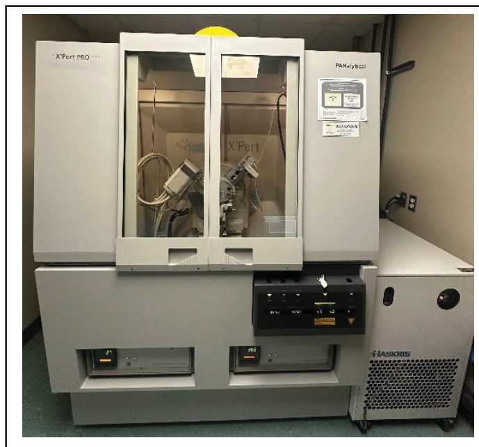
Figure 2-14 X'Pert3 MRD PANalytical X-ray diffraction machine
