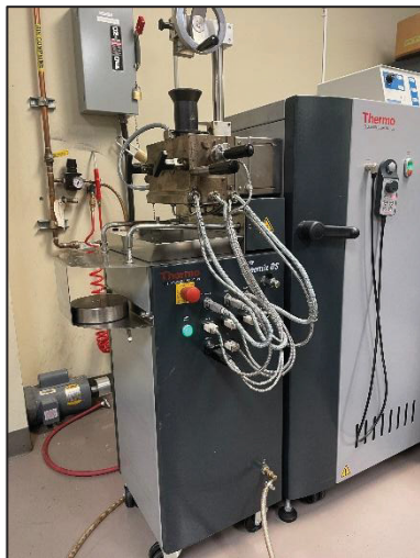
Figure 3.3 Malaxeur interne (Thermo Scientific™ Thermal mixer)
