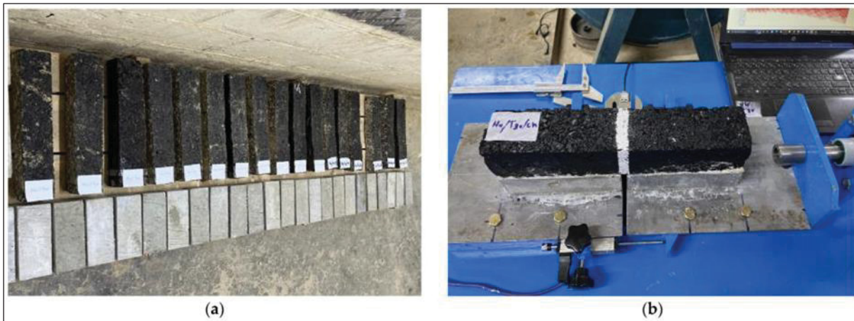
Figure 1.6 Example specimen preparation and overlay testing configuration used to evaluate cracking performance under controlled temperature conditions Taken from Albayati et al., 2023
