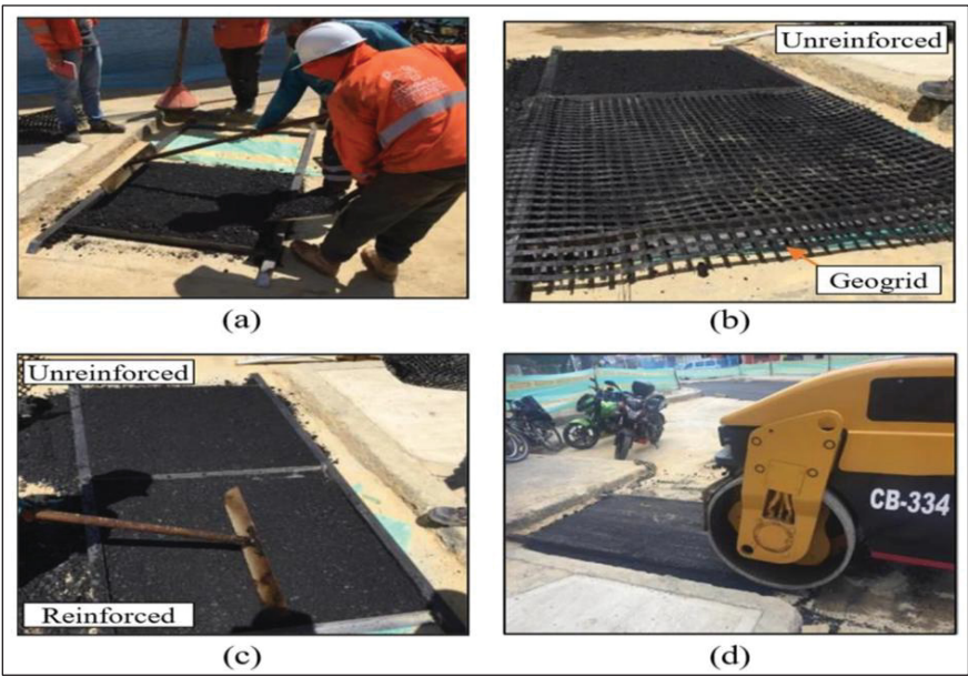
Figure 1.15 Example large-scale slab specimen fabrication and geogrid placement for laboratory evaluation of reinforced asphalt overlays. Taken from Rueda et al., 2023
