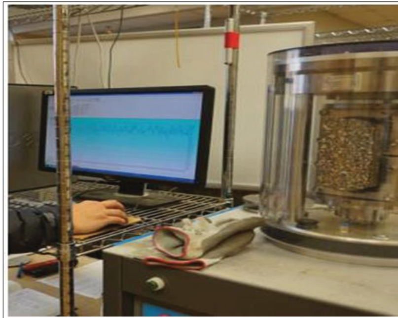
Figure 1.9 Overlay Test (OT) apparatus used to apply cyclic direct-tension displacement to asphalt mixture specimens for evaluating cracking potential.
