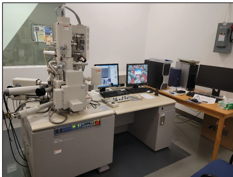
Figure 3-5 The Hitachi SU-70 field emission gun Scanning Electron Microscope (FEG-SEM) setup utilized for microstructural characterization, including Electron Backscatter Diffraction (EBSD) and Energy Dispersive X-ray Spectroscopy (EDS) analysis
