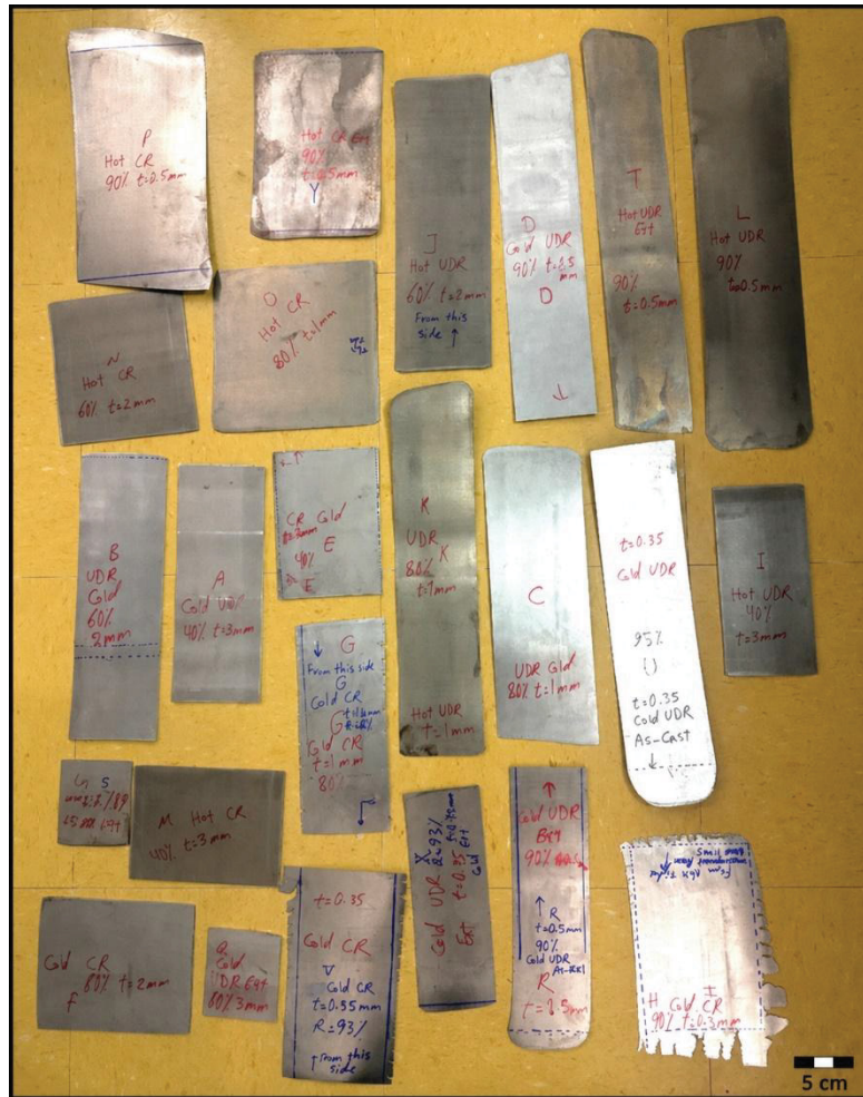
Figure 3-3 Representative examples of plates processed under selected cold and pseudo-hot rolling conditions considered in this study
