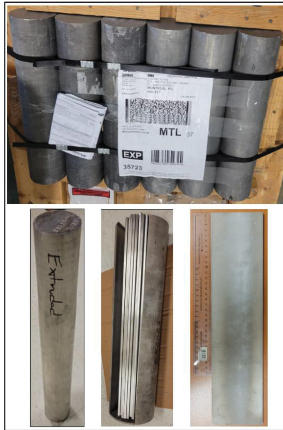
Figure 3-1 Initial materials used in this study, including as-cast AA6063 and AA6082 billets and the as-extruded AA6082 bar, together with examples of longitudinally sectioned and machined plates prepared for rolling
