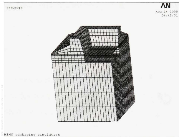
Figure 4.6 Prototype 2 meshing for a cuboid shape package (before its rotation).
