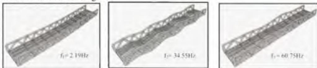
**Figure 4. Finite element analysis of vibration modes.**
