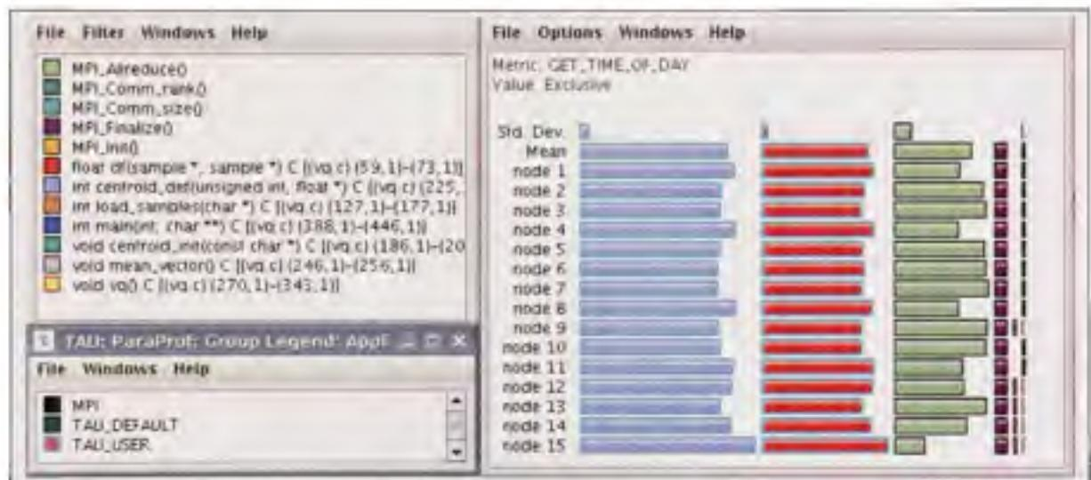
**Figure 2.13 :** Individual functions and group of functions can be selected to focus the displayed statistics. Here, the TAU\_USER group is selected in the *Group Legend* pane (bottom left), which highlights the relevant functions in the main window (right). Note that we have de-selected the stacked bar presentation for the main window to present an alternative to the normalized stacked bars from Figure 2.12 .
