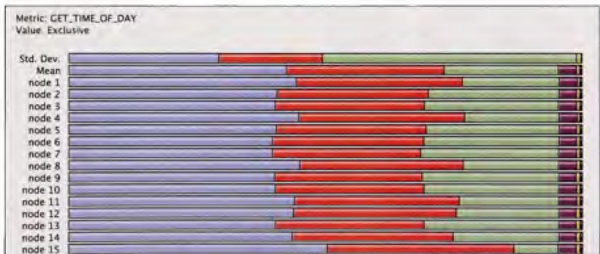
**Figure 2.12 :** A normalized profile view of all processes including the global mean and the standard deviation (Std. Dev.) of each functions. In this case the metric is the time proportion as per `GET_TIME_OF_DAY`. Each color represents a specific function and its length is proportional to the total execution time on that specific node.
