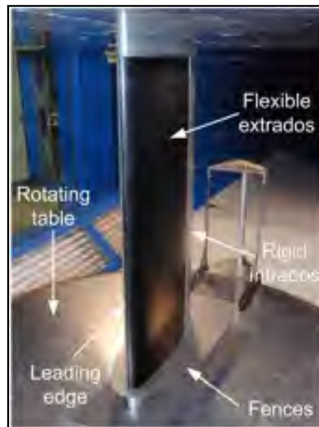
Figure I.7 Morphing wing prototype in the wind tunnel
