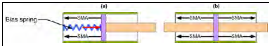
Figure II.1 Schema of SMA actuator with (a) passive and (b) active bias elements
