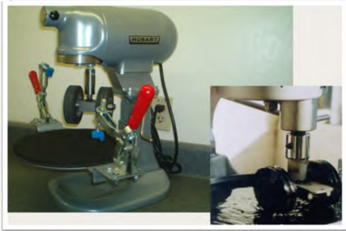
Figure 2.9 Modified wet track abrasion tester Extracted from Slurry/Microsurface - Mix Design Procedure Jim Moulthrop, P.E., (2004, p. 15)
