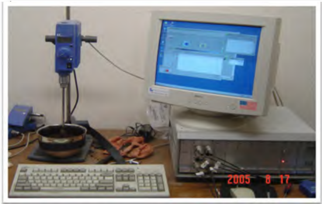
Figure 2.6 German Mix Tester Extracted from Slurry/Microsurface - Mix Design Procedure, Jim Moulthrop, P.E., (2004, p. 15)
