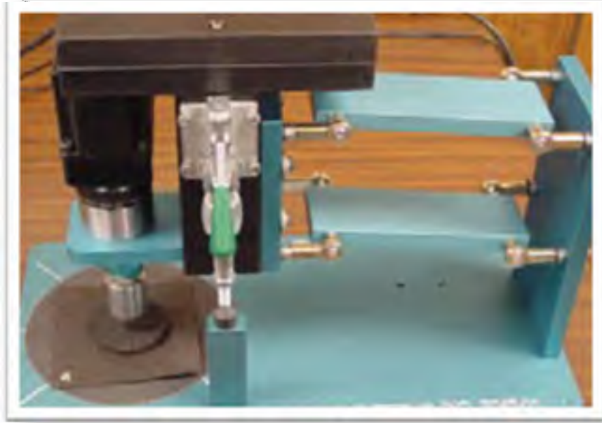
Figure 2.7 Automated Cohesion Tester (ACT) Extracted from Slurry/Microsurface - Mix Design Procedure, Jim Moulthrop, P.E., (2004, p. 15)
