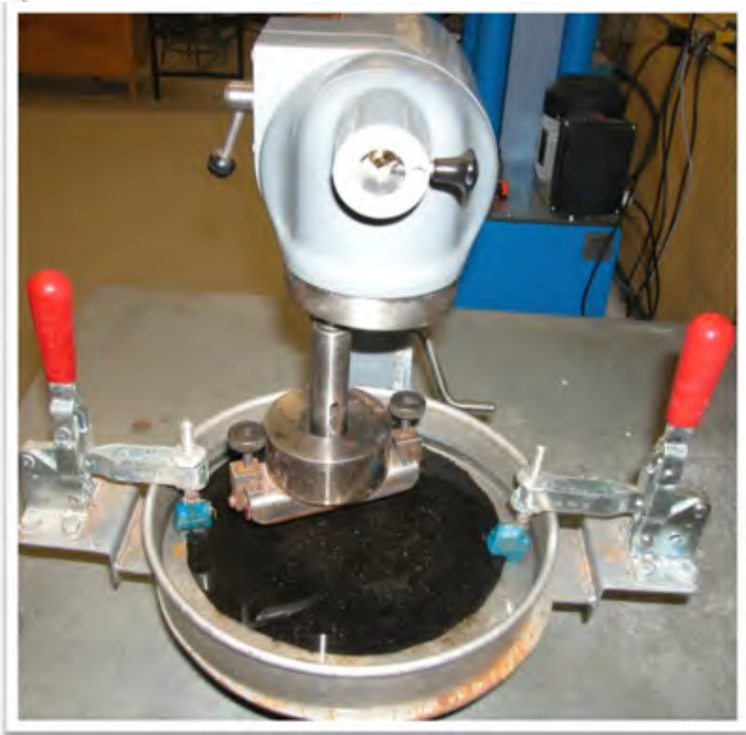
Figure 5.2 Wet Track Abrasion Testing Machine (Hobart N-50)
